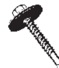
#12-14 x 1-1/4" HWH w/1-1/8" Oversize Bonded Washer (pre-drilling w/oversize holes required on all sheets)
